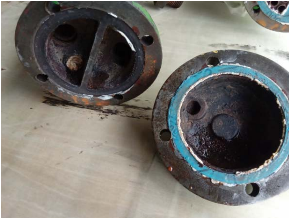
OIL COOLER BEFORE CLEANING
