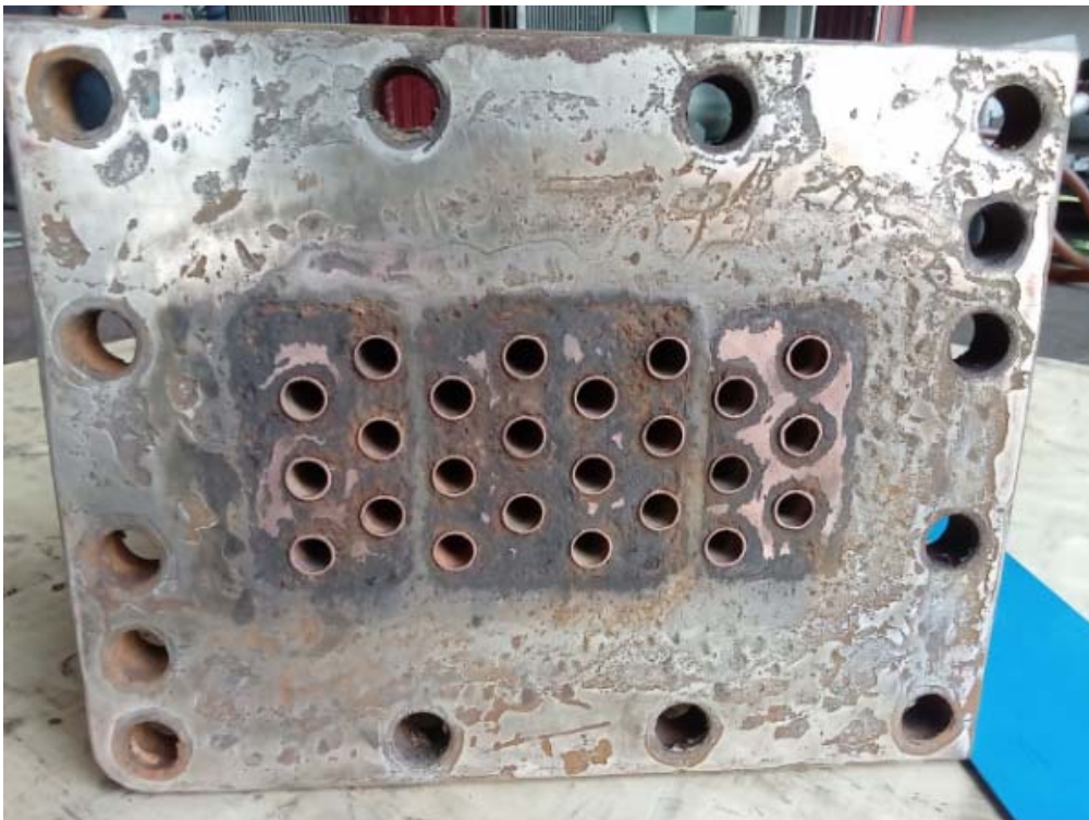
INTERCOOLER AFTER CLEANING
