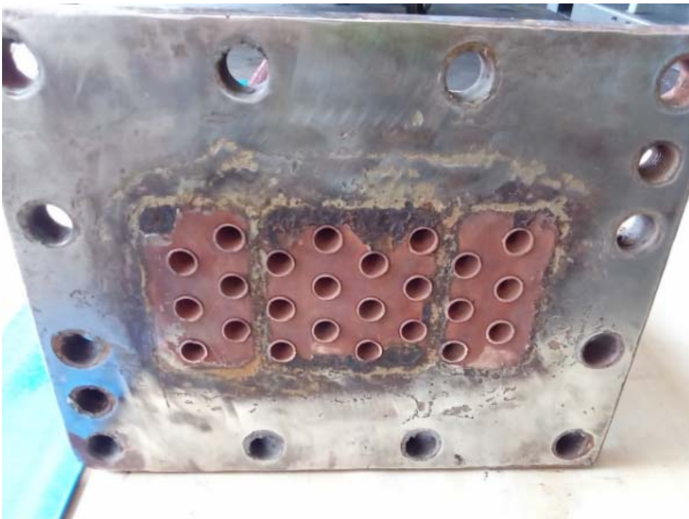
AFTERCOOLER AFTER CLEANING
